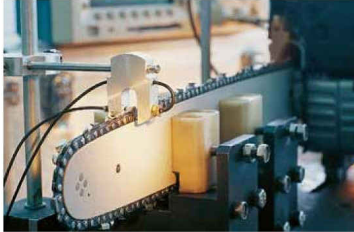
Brake test in our laboratory.
