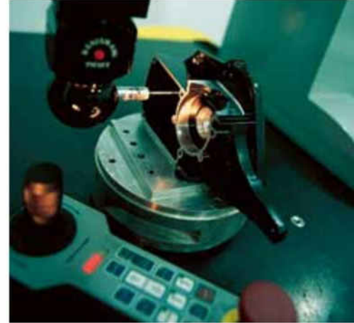
Monitoring the precision of parts on a 3-dimensional measuring equipment.
